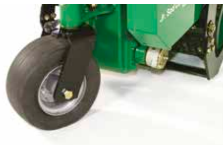
PNEUMATIC SWIVELING REAR WHEEL
