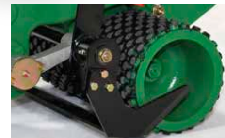
KNOBBY TREAD DRIVE TIRES MOLDED TO HUB
