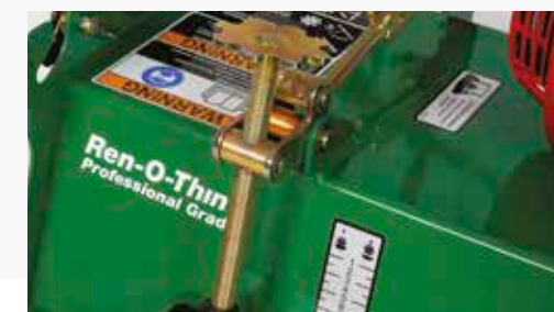
INFINITE DECK HEIGHT ADJUSTMENT
