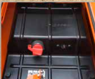
Battery cut-off switch
