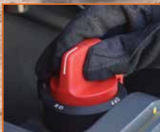
Battery cut-off switch
