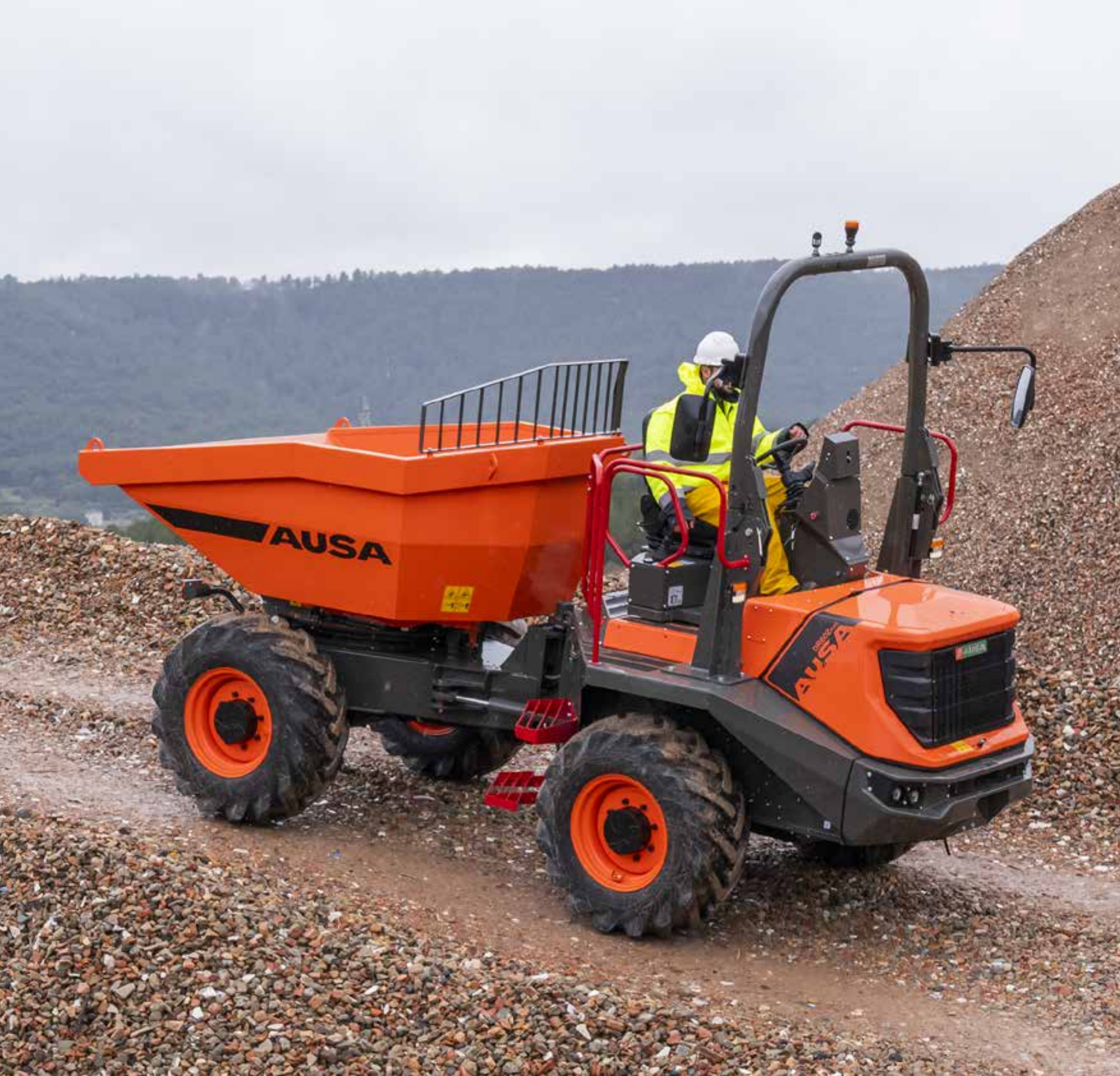
DR602AHG 6000KG UNLOADING SYSTEM SWIVEL TIP POWER 55.4KW WIDTH 2,210MM TRANSMISSION HYDROSTATIC
