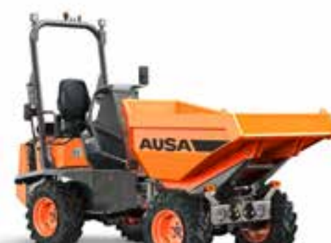
D201AHG 2000KG UNLOADING SYSTEM SWIVEL TIP POWER 18.5KW WIDTH 1,500MM TRANSMISSION HYDROSTATIC
