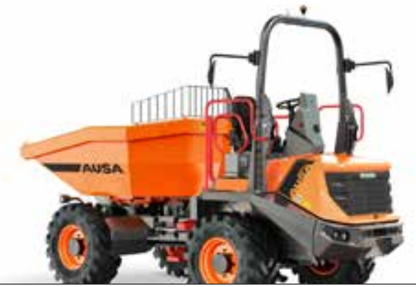
DR602AHG 6000KG UNLOADING SYSTEM SWIVEL TIP POWER 55.4KW WIDTH 2,210MM TRANSMISSION HYDROSTATIC
