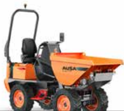
D101AEA 1000KG UNLOADING SYSTEM HIGH TIP POWER 19.6KW WIDTH 1,090MM TRANSMISSION ELECTRIC
