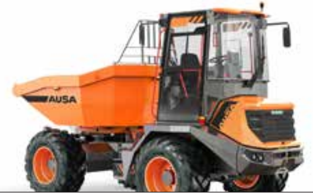
DR902AHG 9000KG UNLOADING SYSTEM SWIVEL TIP POWER 55.4KW WIDTH 2,440MM TRANSMISSION HYDROSTATIC
