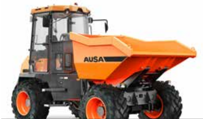
D1001APG 10000KG UNLOADING SYSTEM SWIVEL TIP POWER 55.4KW WIDTH 2,410MM TRANSMISSION TORQUE CONVERTER
