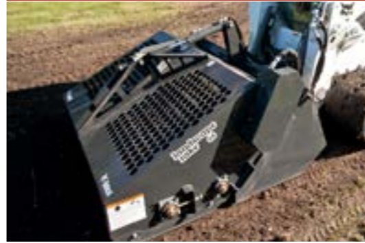
Landscape Rake: Machine must have front hydraulic auxiliary.
