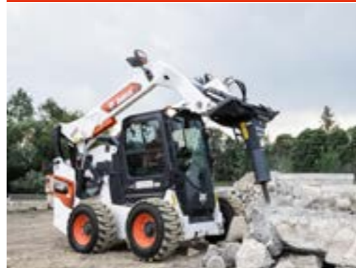
Breaker includes: Nail Point, fixing cap bolts, gauge tool and hose protector. Special Application Kit must be installed on the machine.
