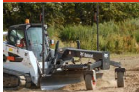
Grader: Loader must be equipped with an Attachment Control Kit.
