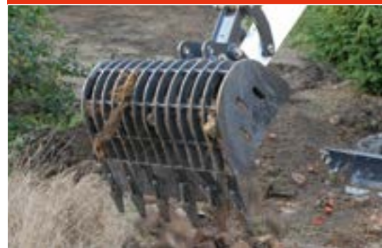
Skeleton Buckets: Type of fittings depends on the coupling system.
