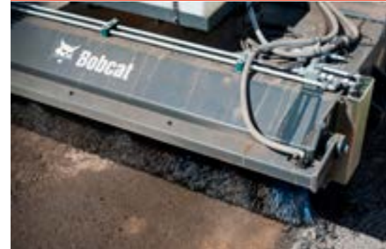
Sweeper: Machine must have front hydraulic auxiliary.
