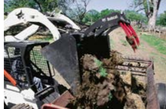
Farm/Utility Grapple: To be attached on bucket.
