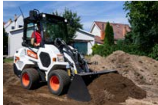
Dirt Buckets: Have predrilled holes to accept bolt-on cutting edge or bolt-on teeth.
