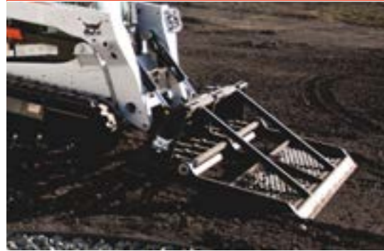
Landplane: Includes expanded metal grate, scarifier assembly, teeth and respective hardware.
