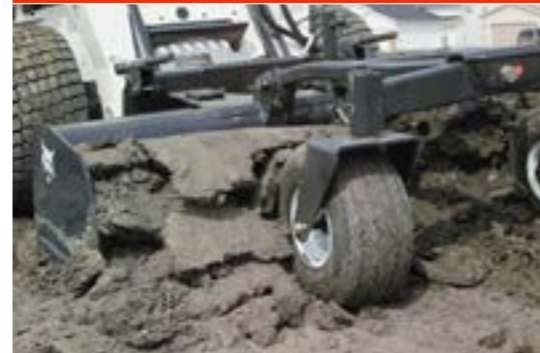
Box Blade: Machine must be equipped with front hydraulic auxiliary.
