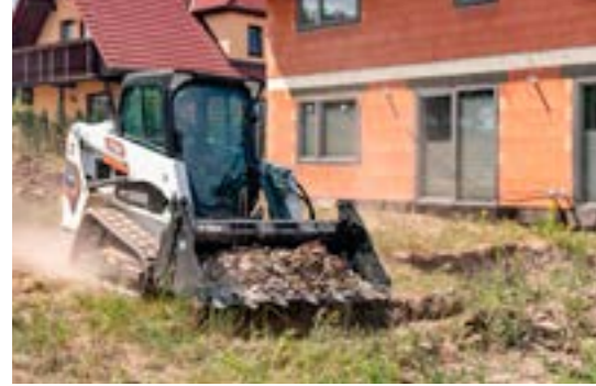
Combination Bucket: It is recommended to use the port relief valve 6684646 for S450/T450 and larger
