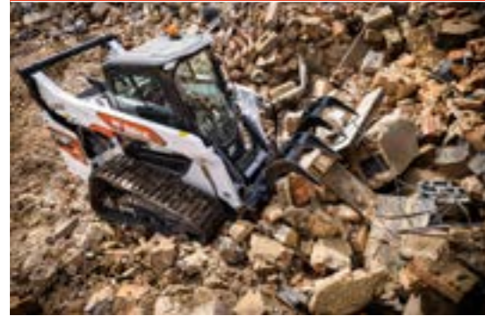
Industrial Grapple: Includes Bolt-On Cutting Edge. It is recommended to use a port relief valve.
