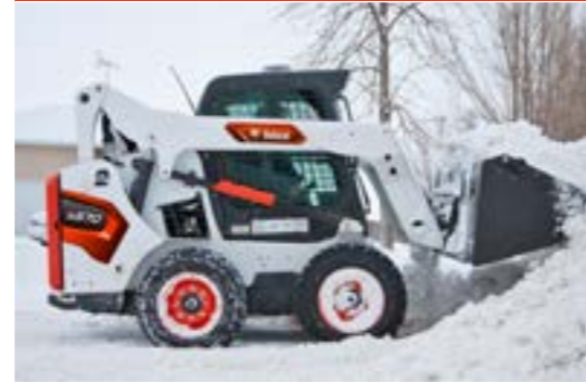
Snow & Light Material Buckets: Have predrilled holes to accept bolt-on cutting edge.
