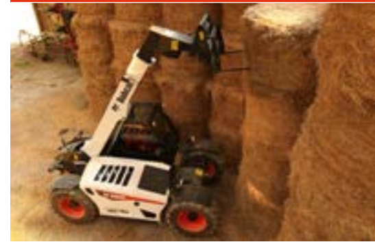
Bale Fork: To be mounted on rigid fork frame.
