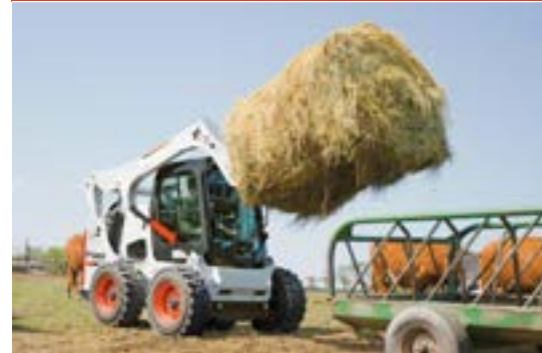
Bale Fork: Need Mounting Frame and Forks.
