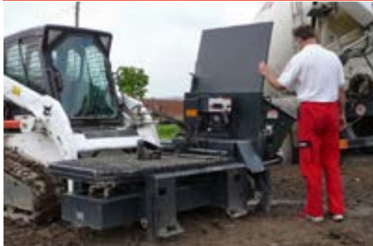
Concrete Pump: Loader must be equipped with an Attachment Control Kit. Attachment includes a 7-Pin Harness only. May also need a Delivery System Kit.
