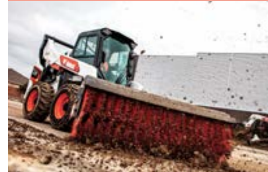
Angle Broom: Loader must be equipped with an Attachment Control Kit.
