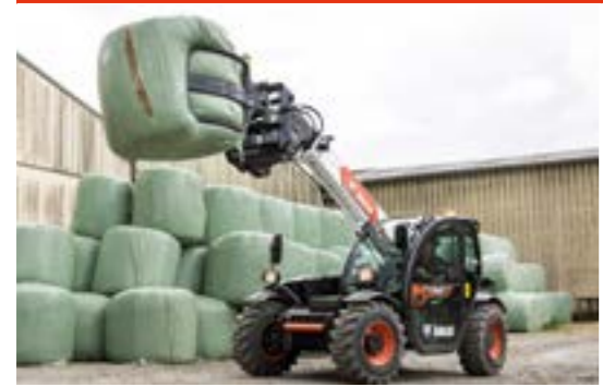
Bale Handler with Tines: Machine must have front hydraulic auxiliary.
