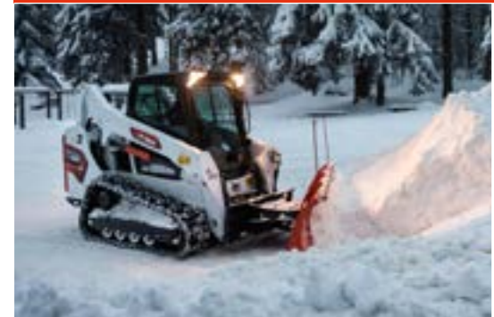
Snow Blade: Includes hydraulic angle
