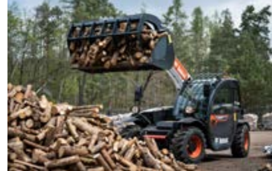
Bucket Grapple: Machine must have front hydraulic auxiliary.
