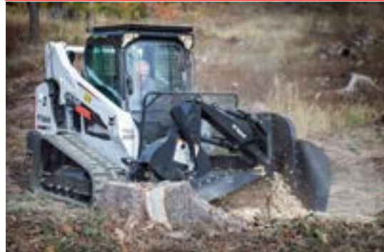
Stump Grinder: Loader must be equipped with an Attachment Control Kit.
