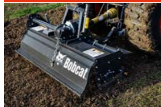
Tiller: Rear-PTO powered 540 rpm.
