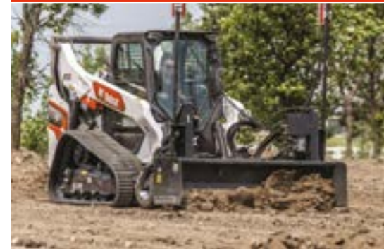
HD Box Blade: Loader must be equipped with an Attachment Control Kit.
