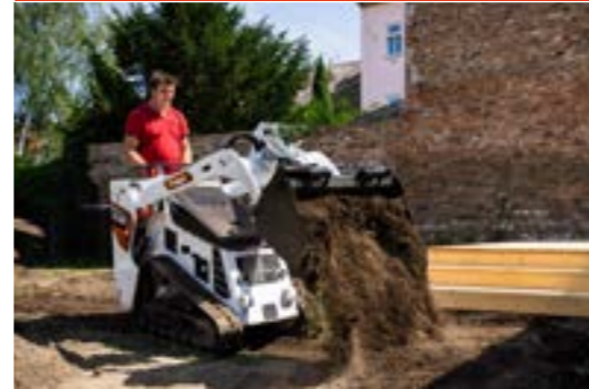
General Purpose Buckets (GP): Have predrilled holes to accept bolt-on cutting edge or bolt-on teeth.
