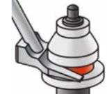
Use Bobcat **6678073**, **6678074** tools for extracting worn bits from attachment when they need to be replaced.
