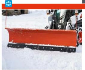
Snow Blade: Included hydraulic angle. Machine must have front hydraulic auxiliary.
