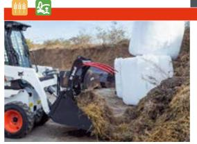
Farm/Utility Grapple: To be attached on bucket. It is recommended to use the port relief valve 7502313. Machine must have front hydraulic auxiliary.
