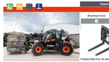
Floating forks are free to swing while remaining level with the ground.
