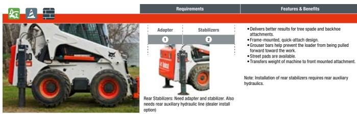
Description: Increase your auger, backhoe or tree spade performance in a wide range of jobs with a set of frame-mounted rear stabilizers. Rear stabilizers improve performance by transferring the weight of the loader to the auger, backhoe or tree spade where it's needed for better digging capability. Rear stabilizers also assist in levelling the loader on uneven terrain. Rear stabilizers are available for most Bobcat loaders and can be quickly mounted and removed.
