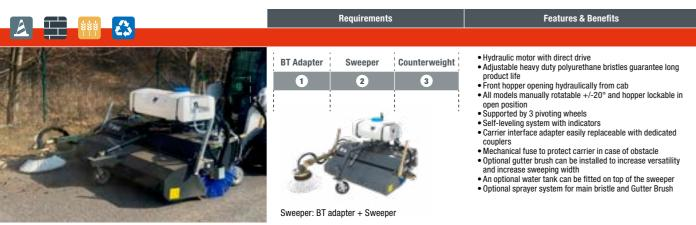
Description: The Bobcat multipurpose sweeper can sweep and collect dirt or other debris. Floating parallelogram self-levelling system guarantee an ease of operation while getting the job done. Angling the sweeper and reversing the flow it can be use for material removal without collection on the hopper. Multiple interface adapter easily interchangeable for each carrier. This attachment is perfect for cleaning parking lots, roads, docks, and warehouses.
