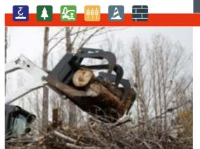
Root Grapple: To be attached on bucket. It is recommended to use the port relief valve 7502313. Machine must have front hydraulic auxiliary.
