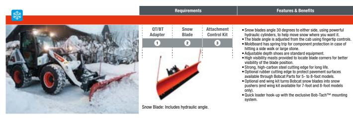
Description: An excellent way to quickly remove light or moderate snow from sidewalks and driveways. Moldboard angles right or left up to 30°. High visibility masts help locate blade corners.
