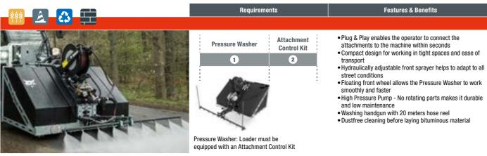
**Description:** The Bobcat Pressure Washer is a versatile attachment that can be used to clean and sanitize streets, remove graffitis and even for railroad, bridge or tunnel maintenance. It's dustfree design enables the attachment to be used when laying asphalt, providing a clean surface for bituminous material laying. Designed to spray high pressured water on roads or any kind of surface that needs to be cleaned. Washing handgun with 20 meters hose reel makes cleaning effective and easy.
