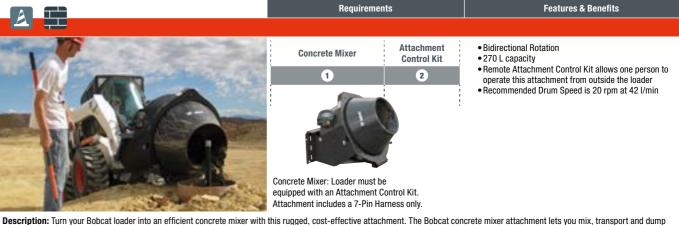
**Description:** Turn your Bobcat loader into an efficient concrete mixer with this rugged, cost-effective attachment. The Bobcat concrete mixer attachment lets you mix, transport and dump concrete much quicker than a traditional stand-alone mixer and wheelbarrow. The attachments compact size makes it perfect for sidewalks, driveways, finish work, and footings and floors of small buildings. It's great for working in hard-to-reach or limited-access areas.
