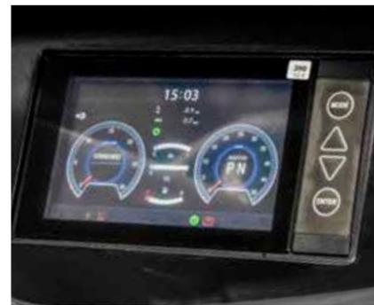
Enjoy a standard 5-inch (optional 7-inch) display panel that is bright, clear, and highly visible outdoors, keeping the operator informed about the machine's conditions.
